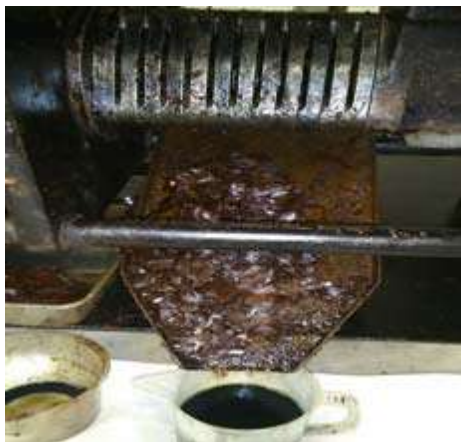
Figure 2.8 Mechanical oil extractions through a screw press
