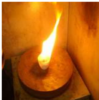
Ash content determination
