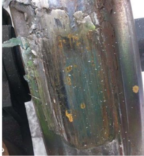
Figure 2.8: Huge freshly made flat, with sheared off material piled up [19]
