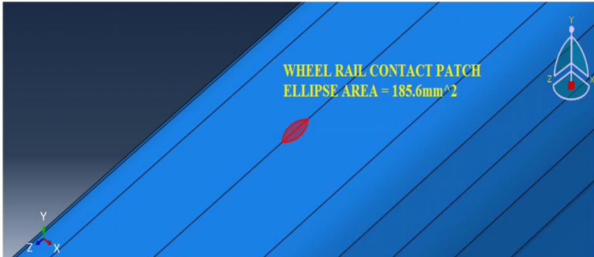
Figure 3.11 wheel-rail contact patch area created by ABAQUS
