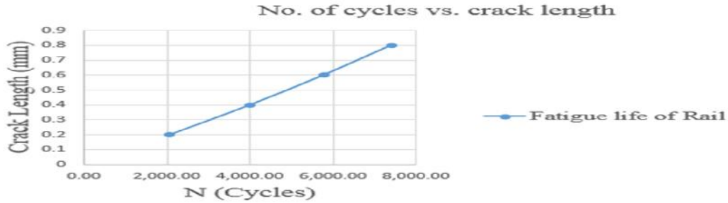
Figure 3.27 Fatigue life of rail (crack at rail head)
