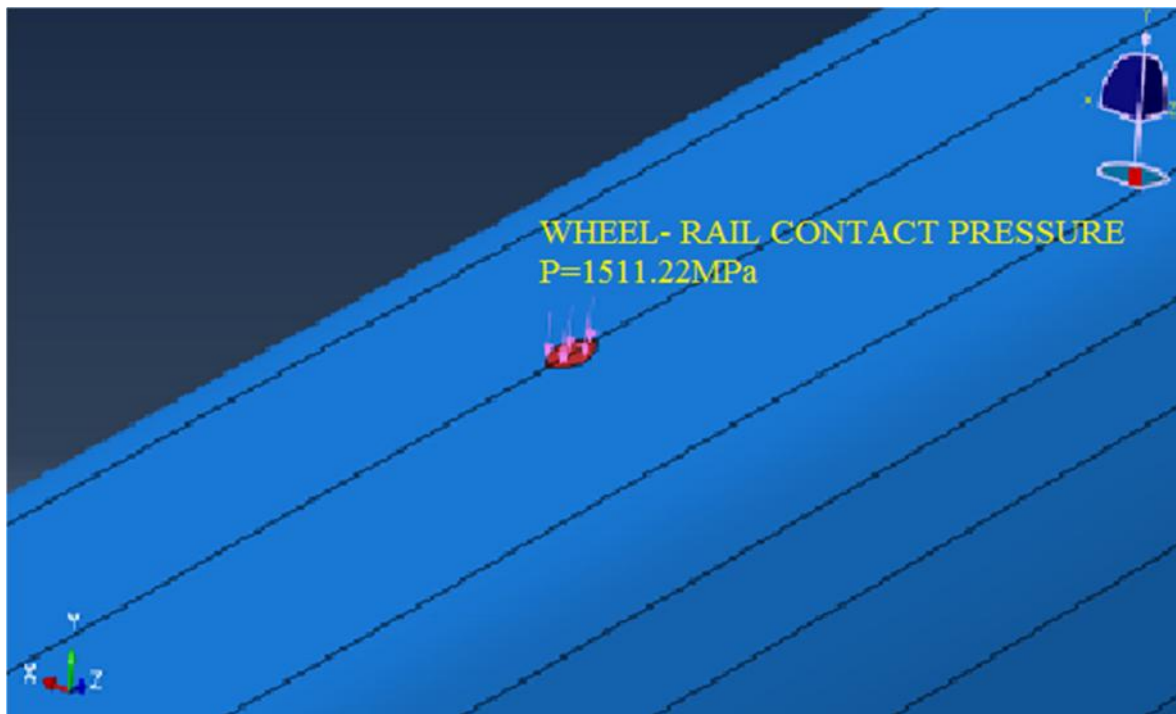
Figure 3.12 loading condition of the rail created by ABAQUS
