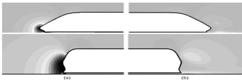
Figure 5: Pressure contours of fore-body and after-body of train: (a) Fore-body of train; (b) After-body of train [89].
