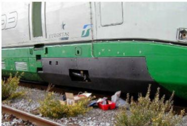
Figure 67: Train with bogie fairings [63].
