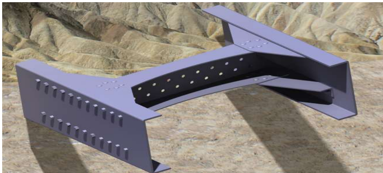
Figuer.3.5.1.9. 3D- Render modeling of existing cross member using CATIAV5R19.
