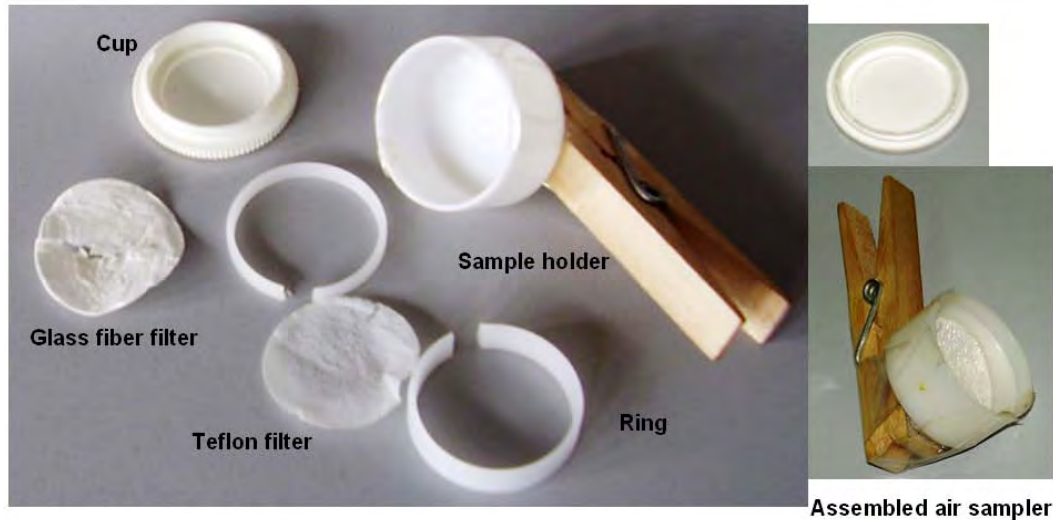
Figure 12: Passive air sampler device and assembling (Willems badge or diffusive sampler)
