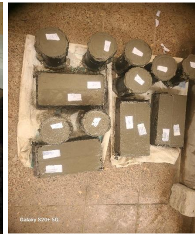
cylinder – absorption and beam-shrinkage
