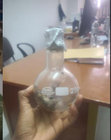
Remaining Aloe Vera pulp after water absorption takes place by freeze-drier
