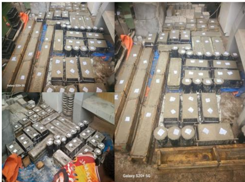
Figure 3.9 Cube, cylinder and beam casted samples
