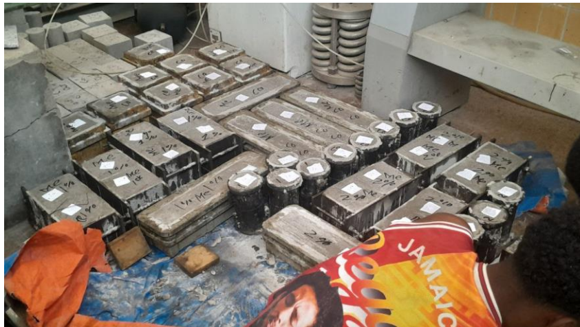
Casted concrete cube, cylinder and beam
