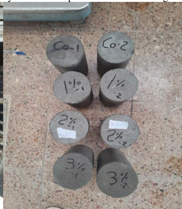
Concrete cylinder for absorption capacity testing at the 28 th day, oven dried for 72hrs.
