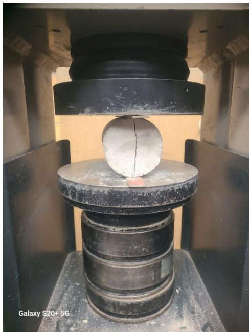
Split Strength testing machine cylinder sample
