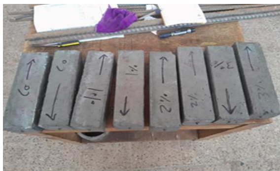
Final Setting time Specimen at the time of No Impression
