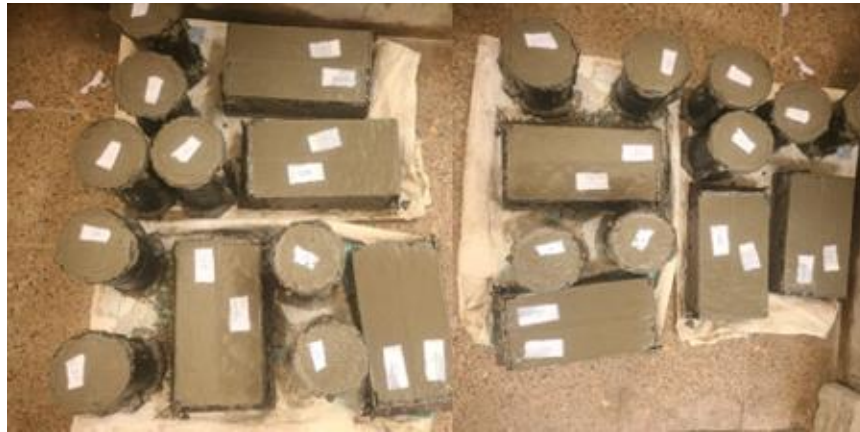
Figure 3.10 Beam and cylinder casted samples for absorption and shrinkage testing
