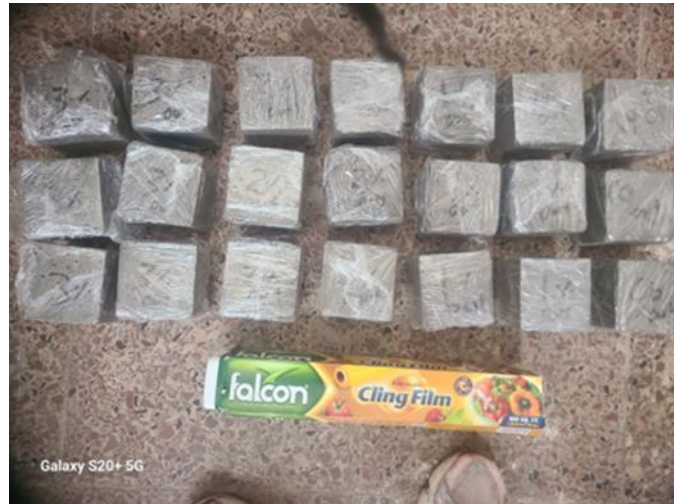
Figure 3.8 Sealed sealed-cured samples
