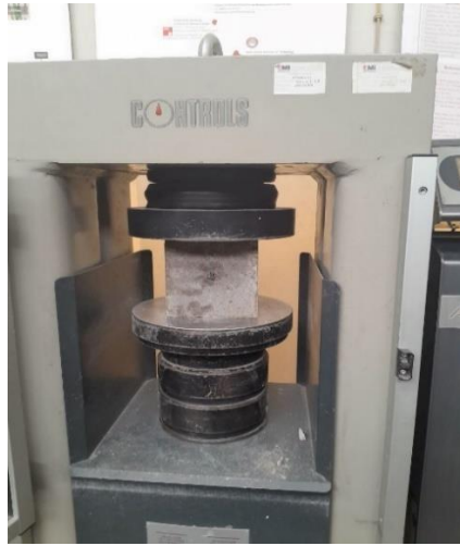
Figure 3.12 Cube sample in compression testing machine
