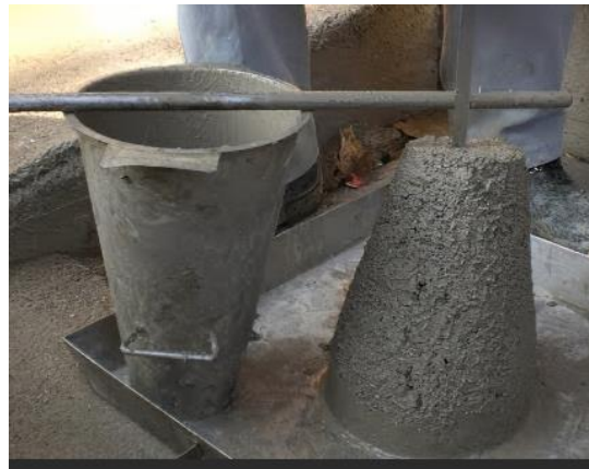
Figure 3.11 Slump test of concrete
