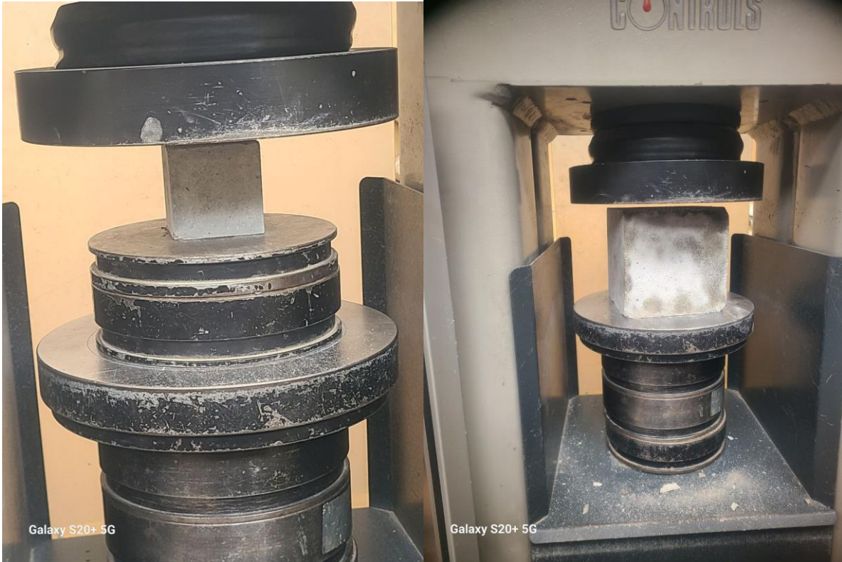
Compressive Strength testing machine and mortar and concrete cube samples
