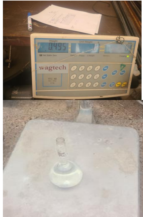
pycnometer filled with water
