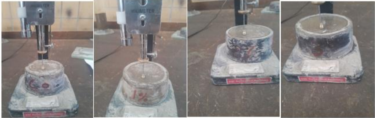
Final Setting time Specimen at the time of No Impression
