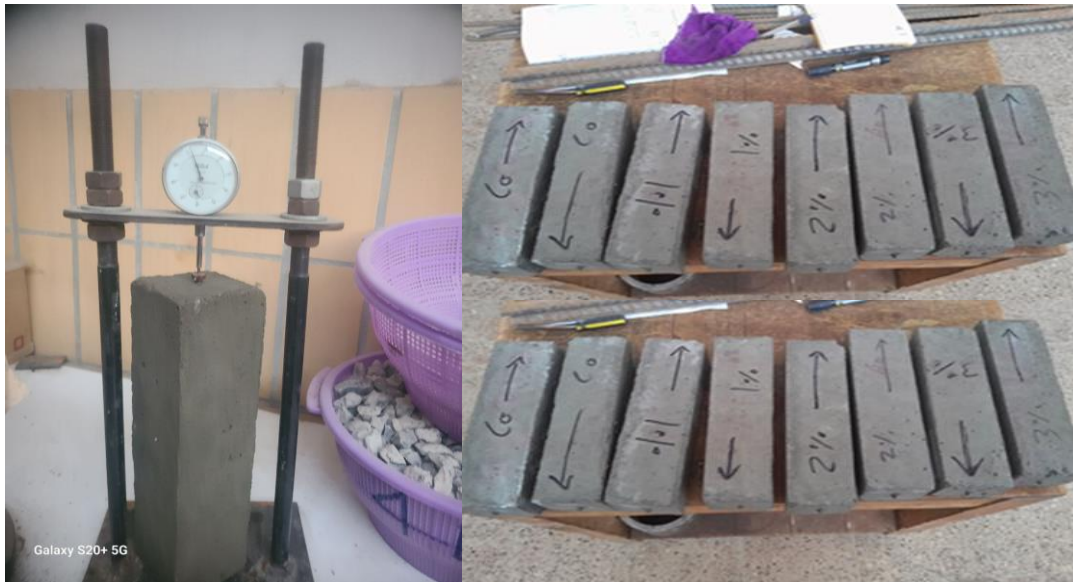
Figure 3.13 Sample beams for drying shrinkage testing
