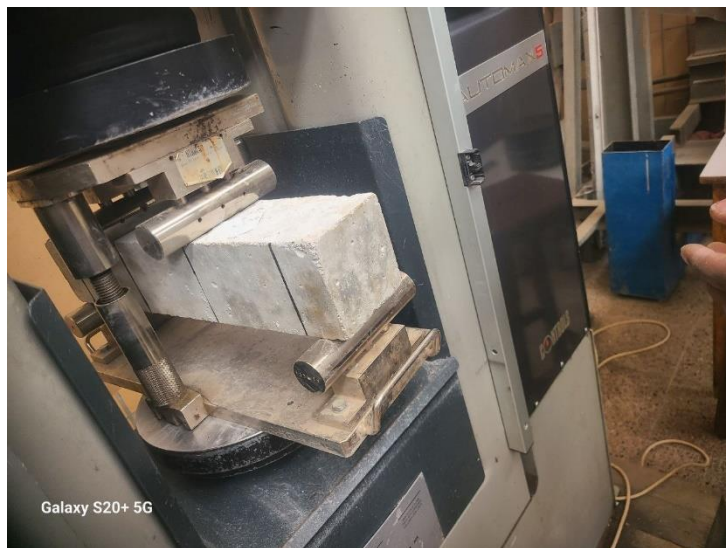
Flexural Strength testing machine a beam sample
