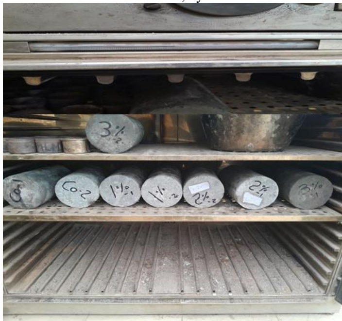
Concrete cylinder for absorption capacity testing at the 28 th day, oven dried for 72hrs.
