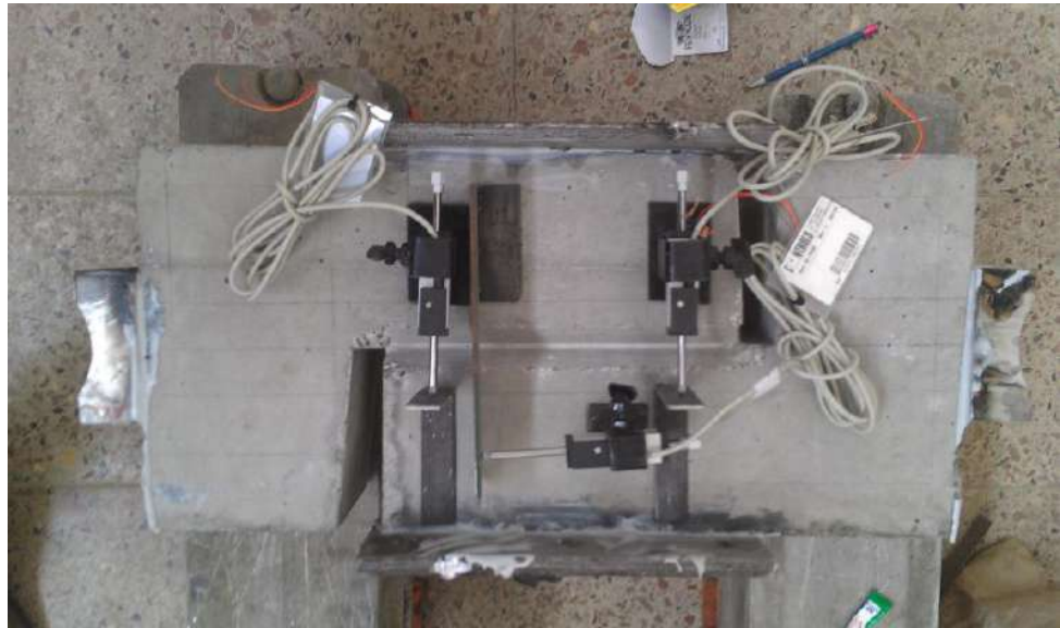
Figure.3. 5: Attaching transducers to the sample
