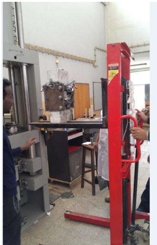
Figure.3. 6: Placing the sample in the universal compression machine for testing
