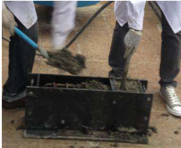
Figure.3. 2: Casting of Push off Sample
