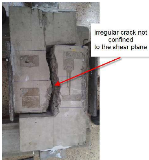
Figure.4. 4: Sample type b failure
