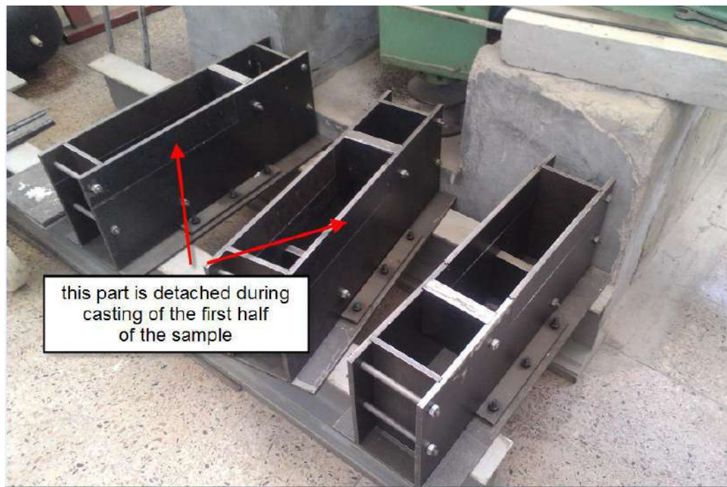
Figure.3. 1: Steel formwork used for preparing push off samples
