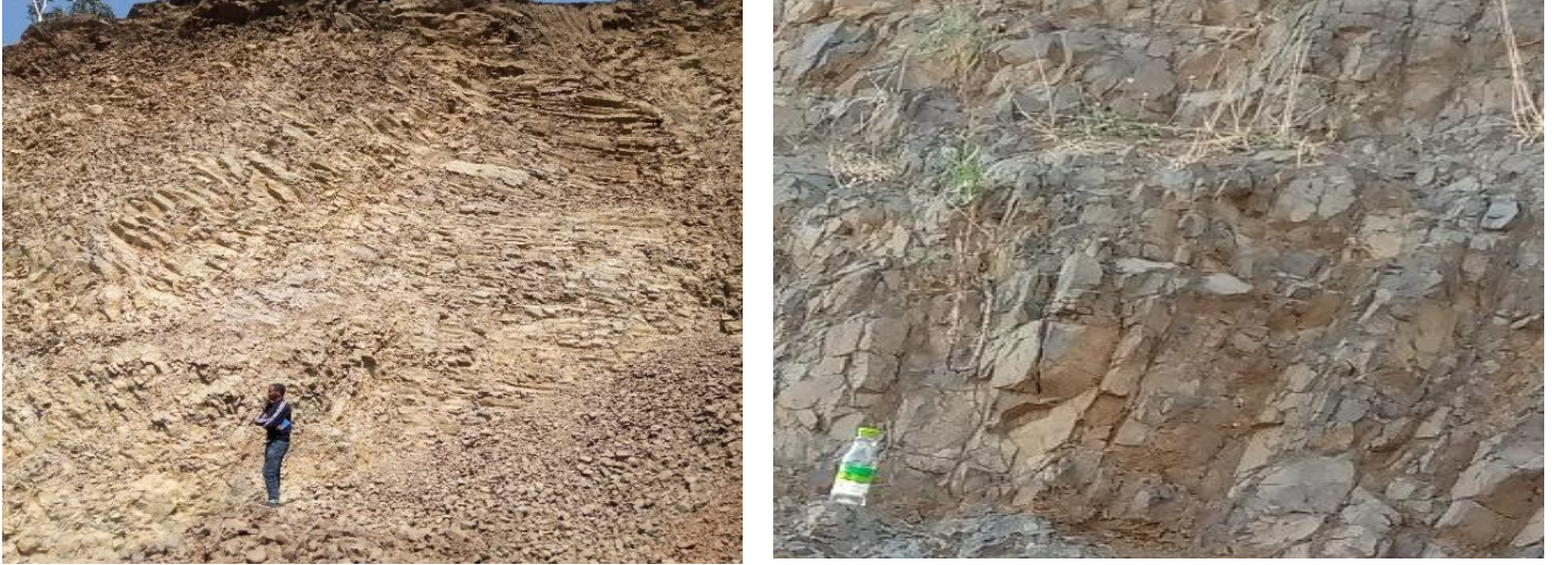
Plate 1: Highly weathered and fractured Ashange basalt exposed to the east of Wuchale (left) and near Lake Hayk (right).
