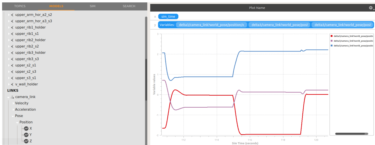
Figure 4-6: Delta 3 robot end effector position at a given time interval
