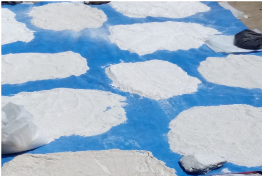
Figure 3.3: Gypsum powder samples during air drying at room temperature
