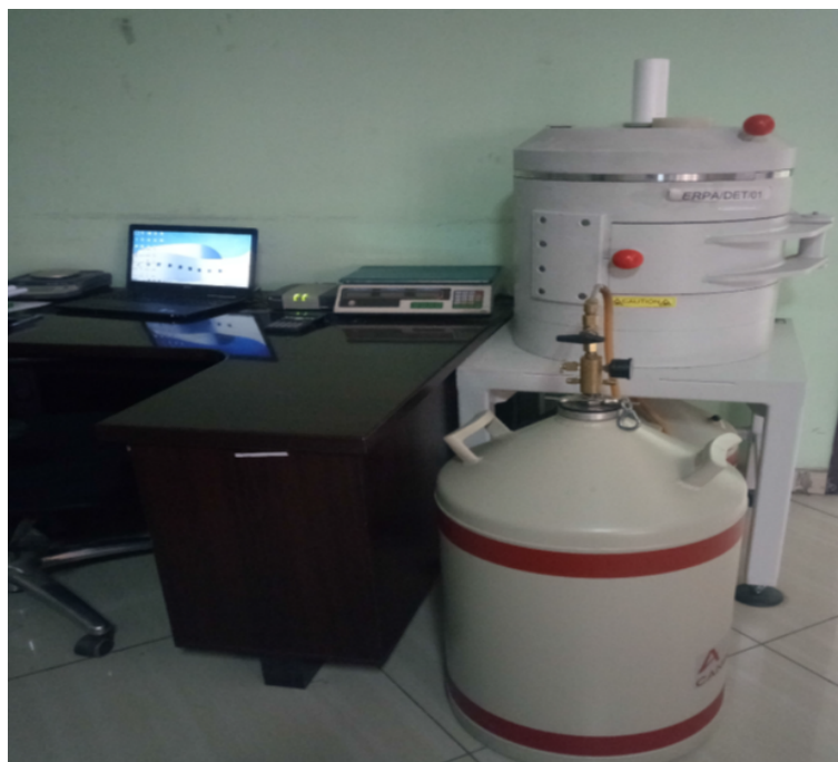
Figure 3.9: Experimental setup of a HPGe detector at ERPA laboratory
