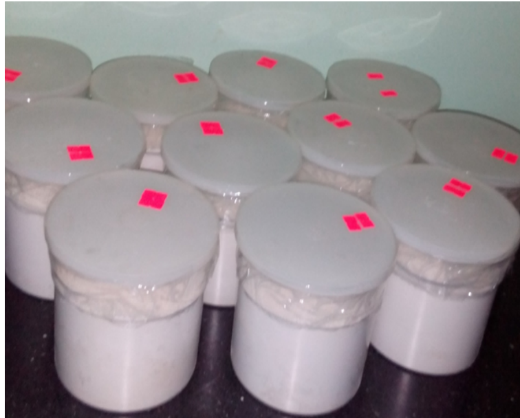
Figure 3.6: Prepared samples sealed in Marinelli cups in ERPA laboratory
