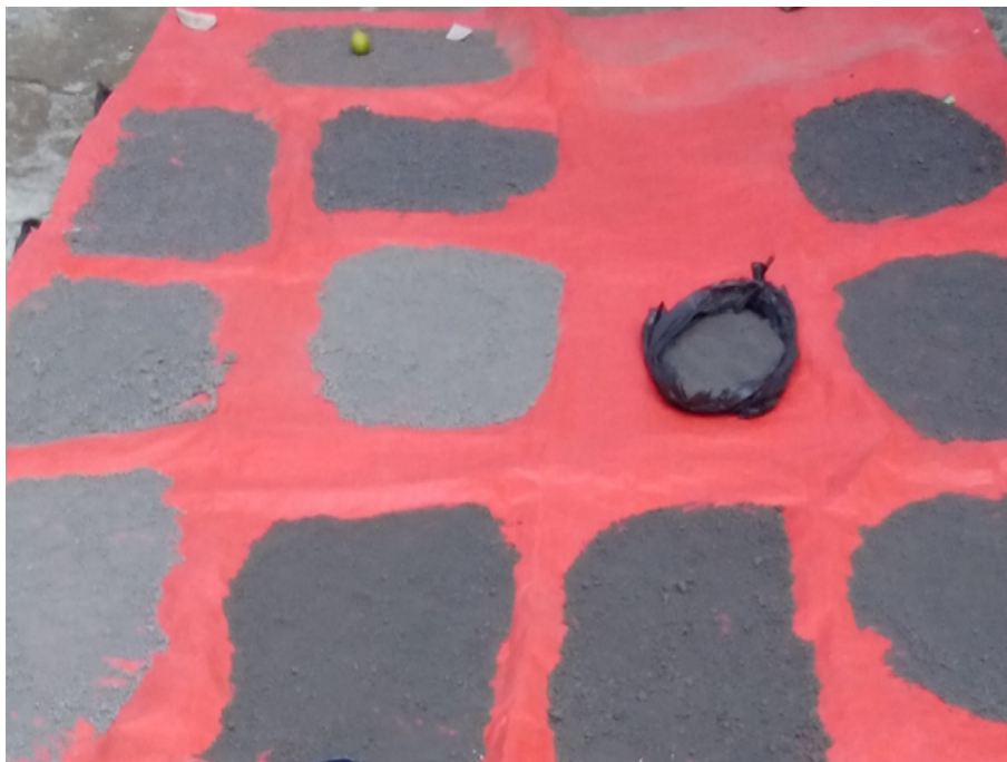
Figure 3.4: Crushed soil samples during air drying at room temperature
