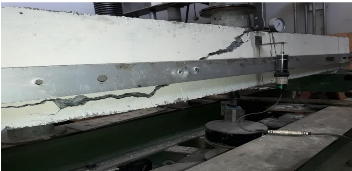
Figure 5.2: FCB75 after failure (front side)
