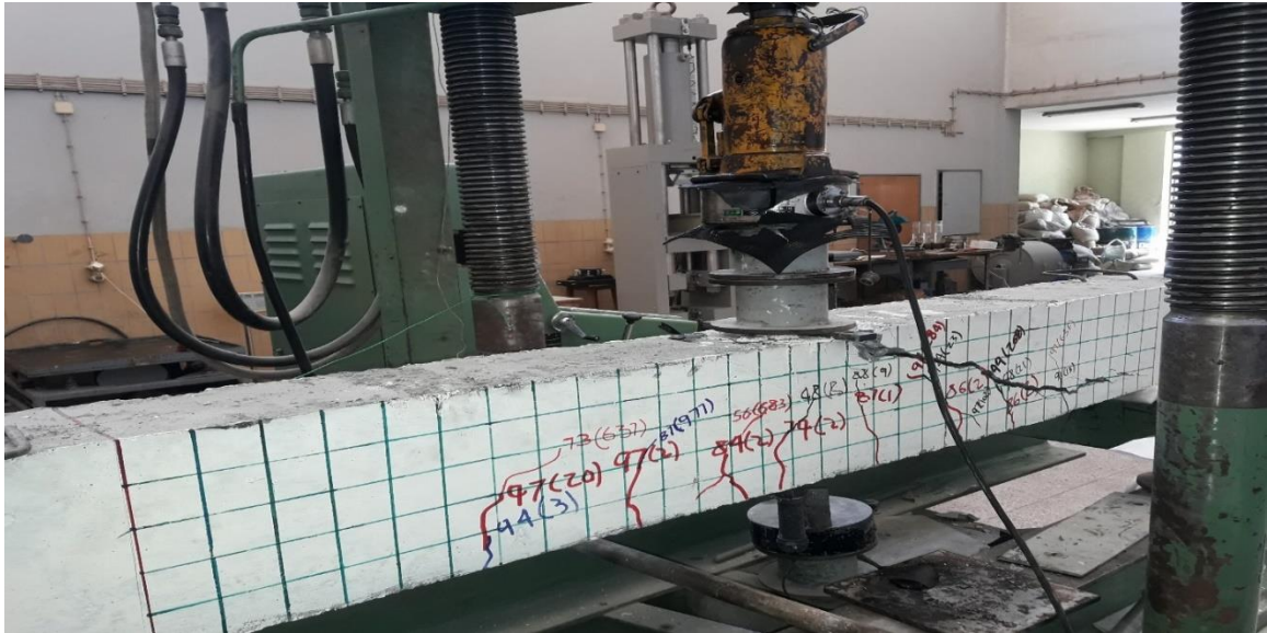
Figure 5.2: FCB75 after failure (front side)
