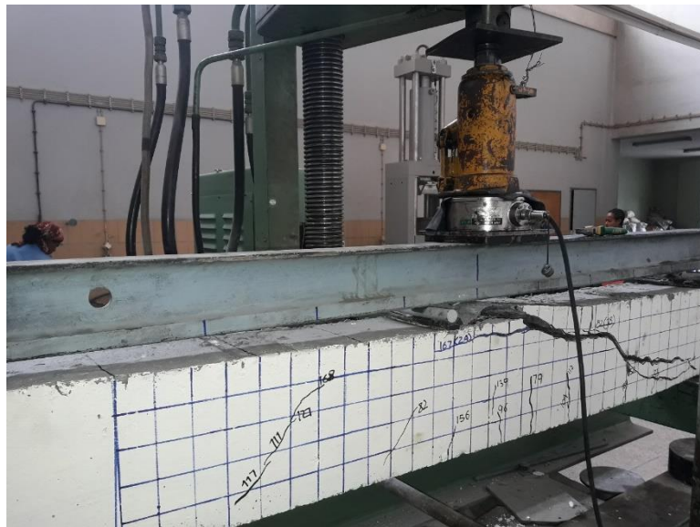
Figure 5.6: MCB85 after failure
