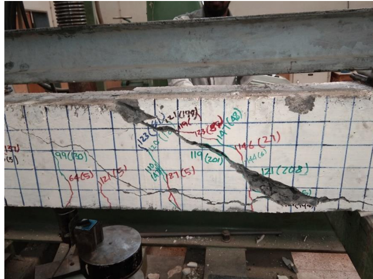
Figure 5.8: MCB75 after failure
