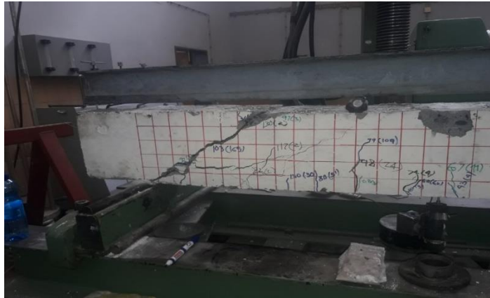
Figure 5.10: MCB68 after failure
