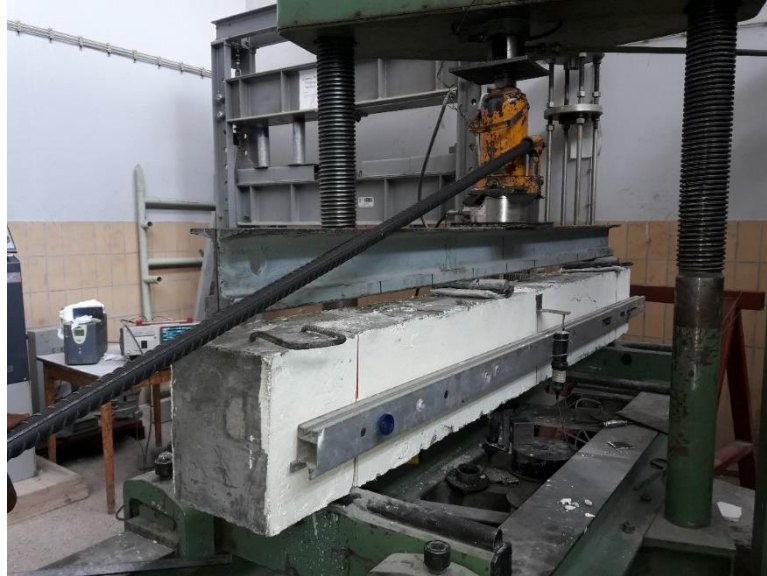
Figure 3.12: linear variable displacement transducers (LVDT) installed at the back
