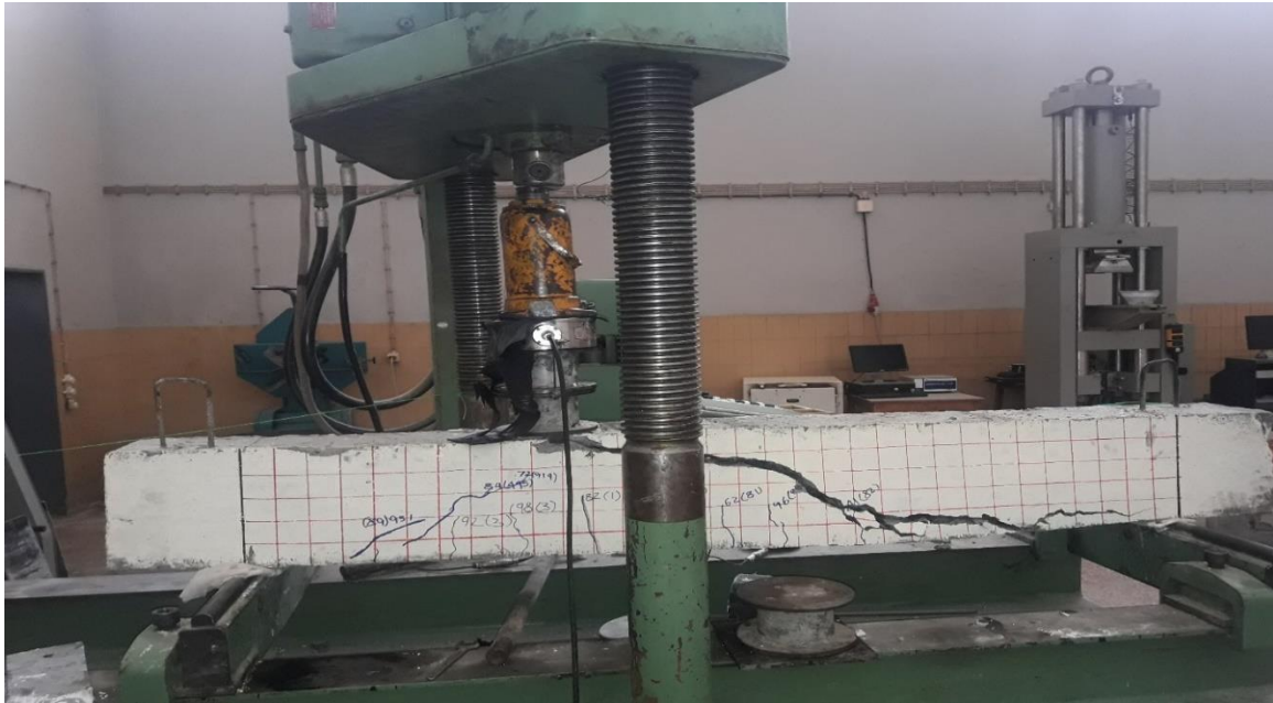
Figure 5.4: FCB75c after failure
