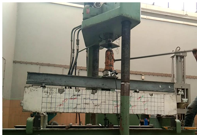
Figure 5.7: diagonal cracks propagating in to compression zone in both halves of MCB75
