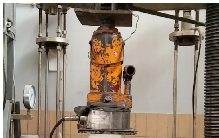
Figure 3.9: hydraulic jack and load cell
