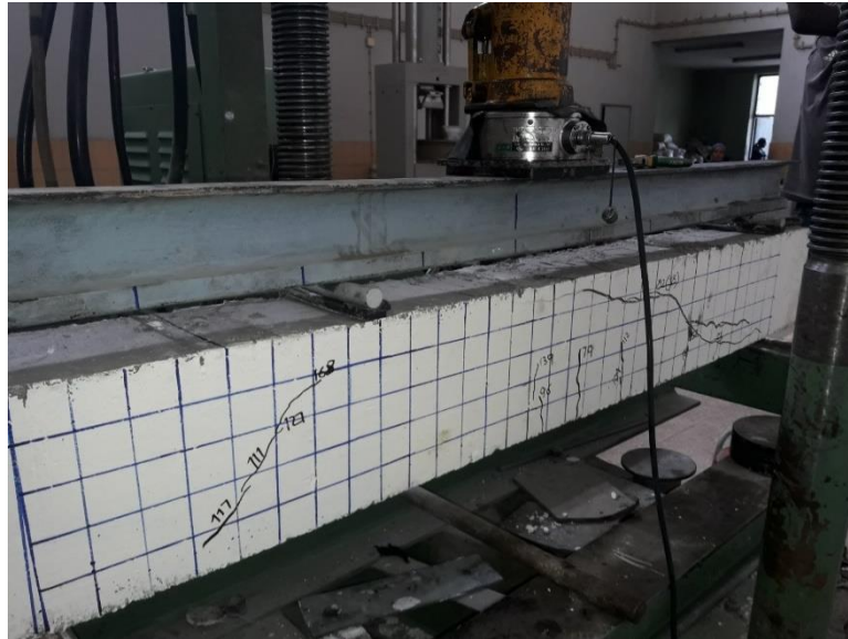
Figure 5.5: Diagonal cracks in both halves of the specimen MCB85
