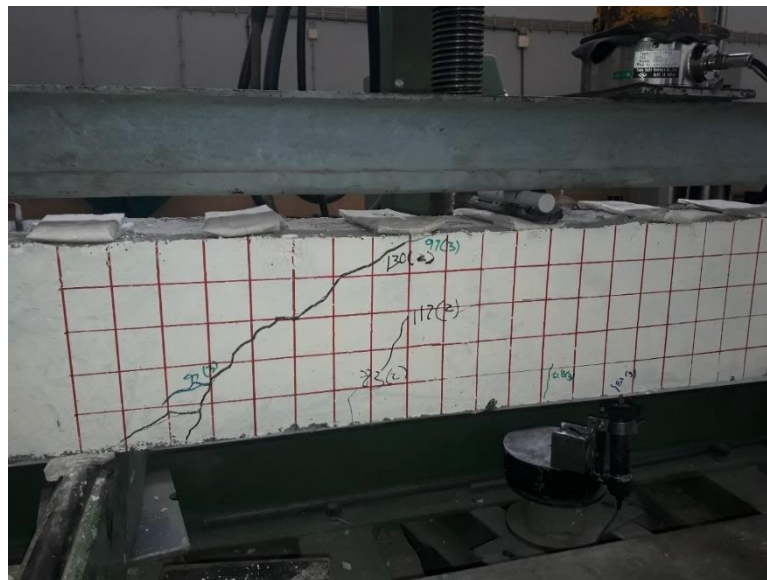
Figure 5.9: diagonal crack that formed in the 2 nd loading in specimen MCB68
