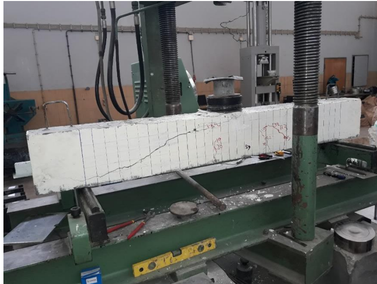
Figure 5.1: MB after failure
