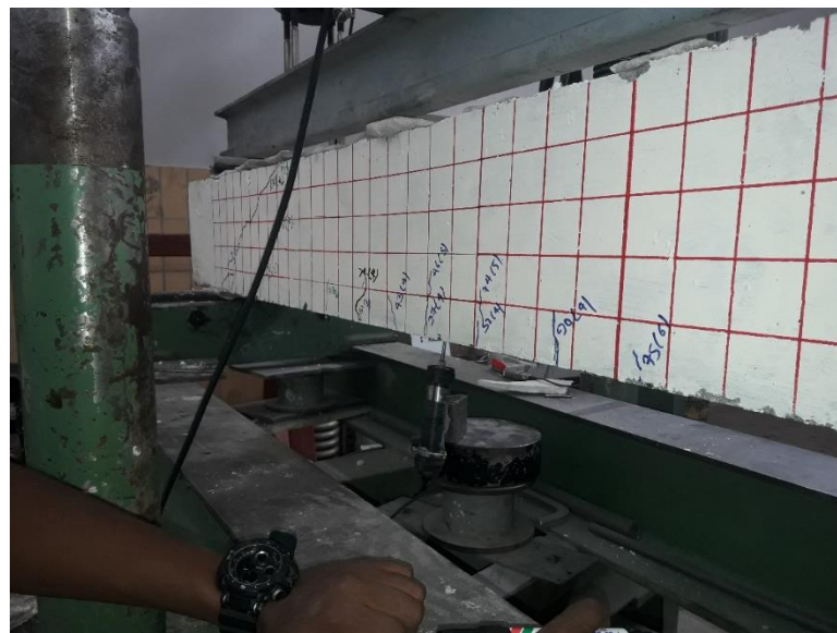
Figure 3.11: linear variable displacement transducers (LVDT) installed under the beam
