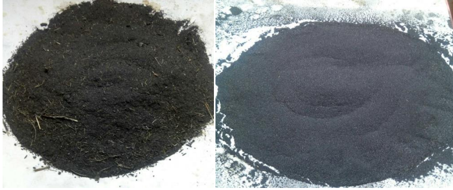
Fig 3.1 Bagasse ash before (left) and after (right) sieving with 250 µm sieve
