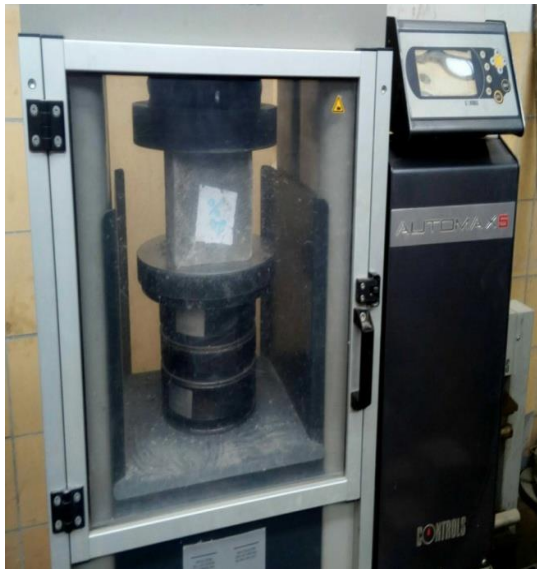
Figure 3.2 Concrete compressive strength tests
