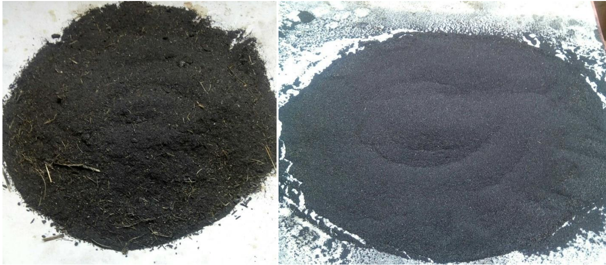
Photo 1 Bagasse ash before and after passed 250 µm size sieves
