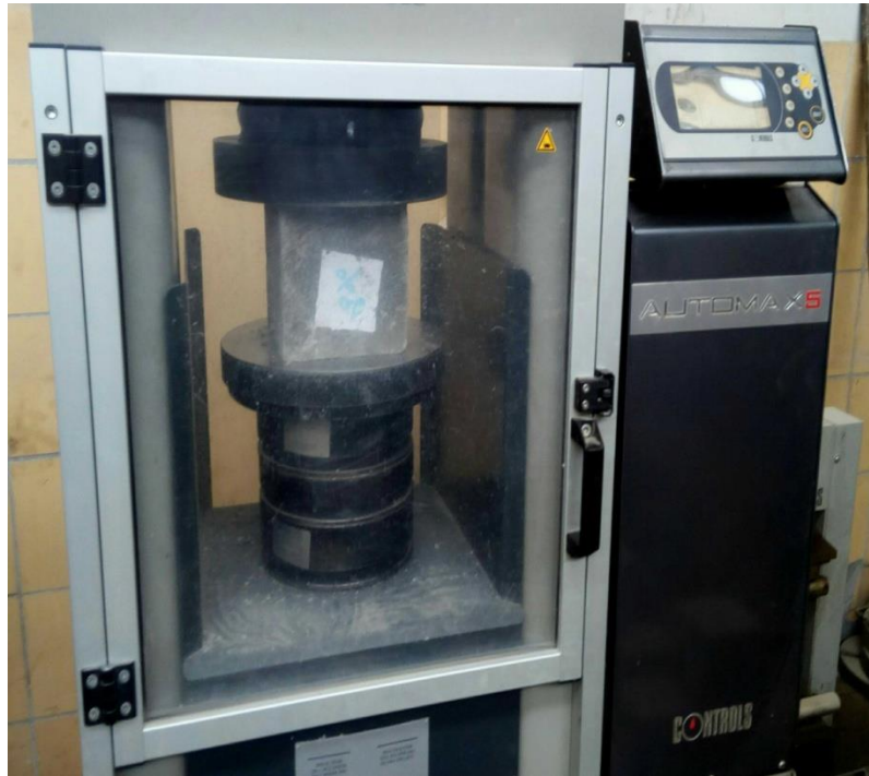
Photo 5 Concrete compressive strength test
