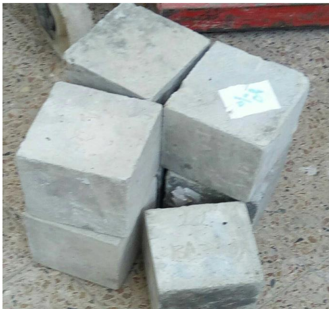
Photo 6 concretes before and after compressive strength test
