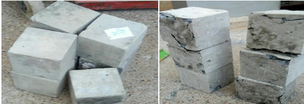
Figure 4.2 Specimen before (left) and after (right) testing compressive strength
