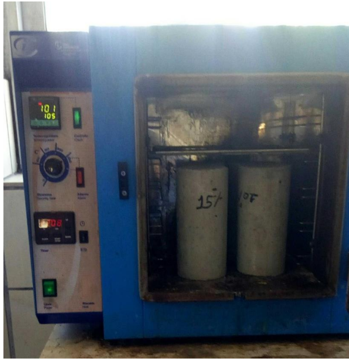
Photo 7 cylindrical concrete in oven dryer
