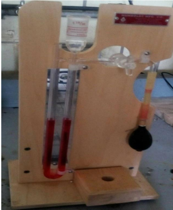
Photo 3 Blain air permeability apparatus
