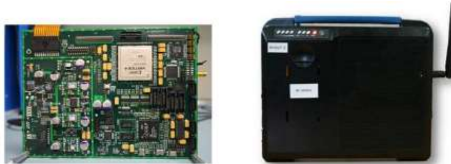
Figure 2.14: FlashLinQ Prototype Modem [88].
