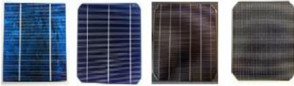
Figure 9 Evolution of standard c-Si cell contacting from 2 bus-bars, 3 bus-bars to 6 bus-bars and ultimately the Smart Wire concept.
