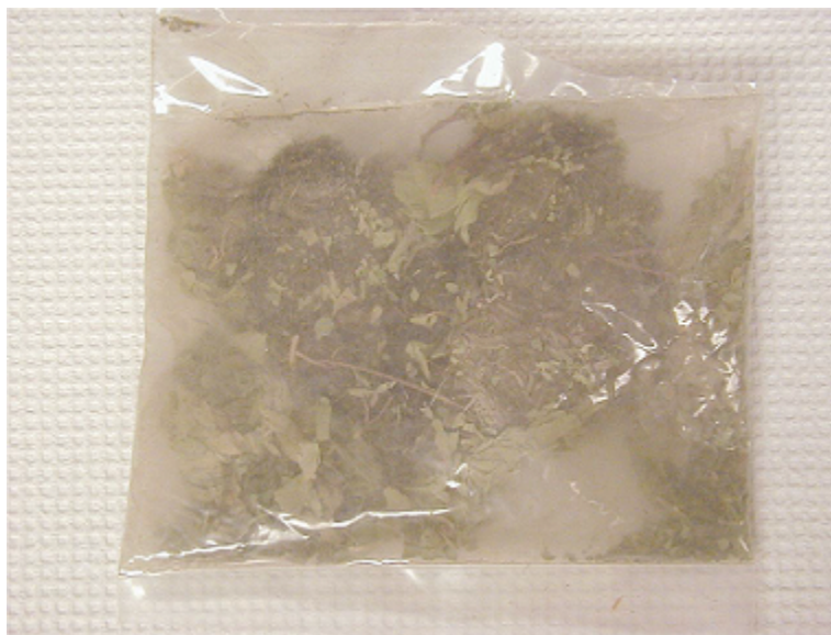
Figure 3.11: Pre-irradiation sample packing by polyethylene films
