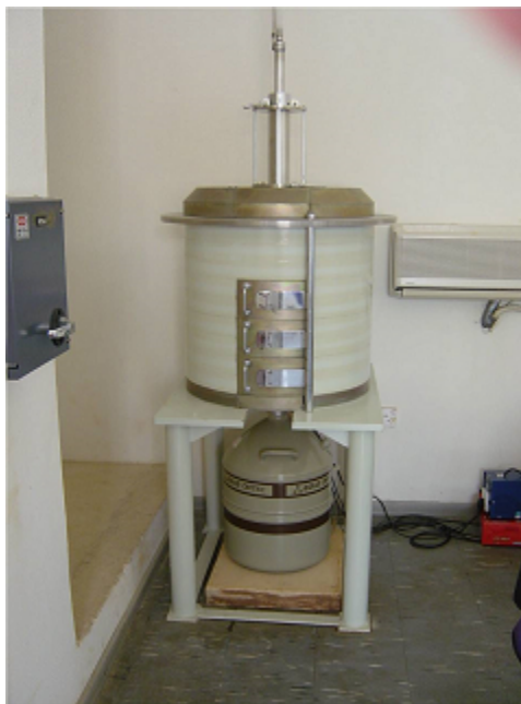
Figure 3.3: GEM70-S detector mounted on 30-liter liquid nitrogen Dewar and enclosed by lead shield
