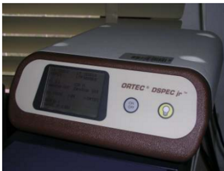
Figure 3.4: Digital Signal processing module, DSPEC jr 2.0
