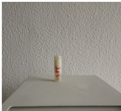
Figure 3.5: Vial container used for packing samples
