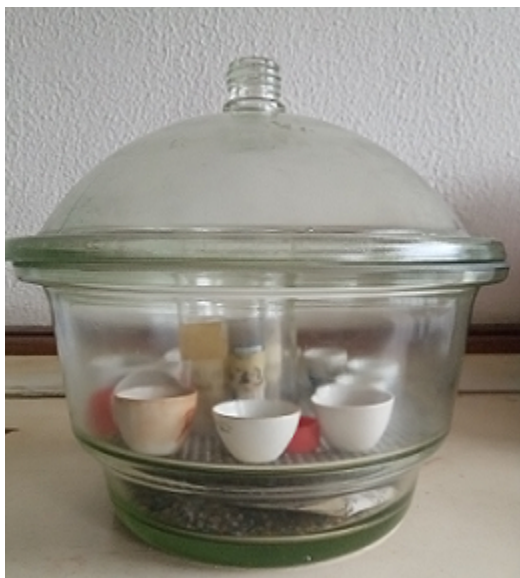
Figure 5.2: Desiccator used for storing prepared samples for irradiation
