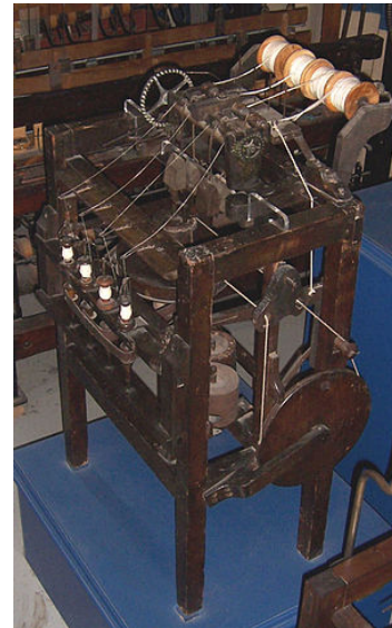
Figure 2.9 The only surviving example of a spinning mule built by the inventor Samuel Crompton
