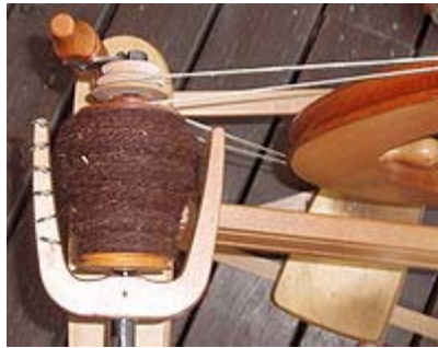
Figure 2.5 A double drive wheel
