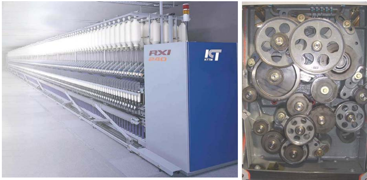
Figure 4.1 Ring spinning machine with its driving mechanism
