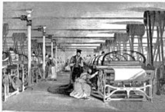
Figure 2.12 A Roberts's loom in a weaving shed in 1835. Note the wrought iron shafting, fixed to the cast iron columns
