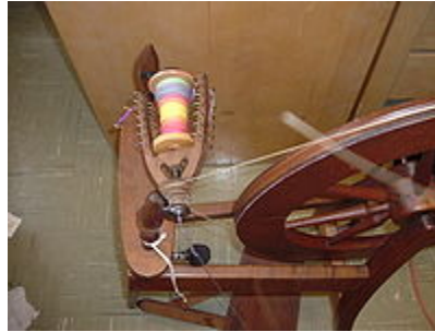
Figure 2.6 A single-drive wheel with the drive band around flyer and brake on the bobbin
