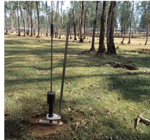
Addis Alem DCP test
