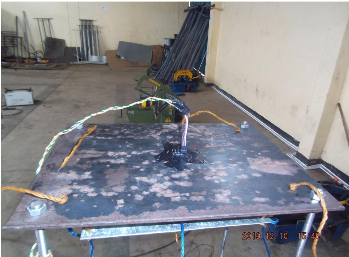
Figure B-4: Gyro accelerometer attached to the top story for taking the data.
