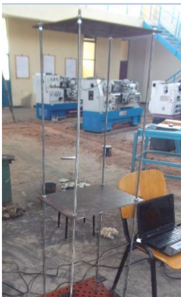
Figure 3.8. Photographs of the two masses at which the model was tested – 14.104kg and 14.7kg respectively.
