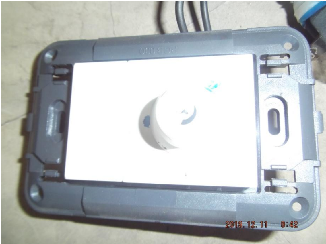
Figure B-6: Dimmer Switch for controlling the speed of the Hammer Drill.
