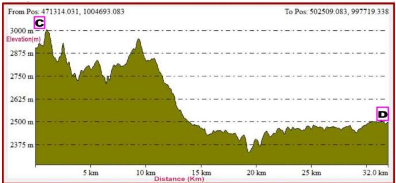
b) Cross sections of the study area along the line C- D on the DEM
