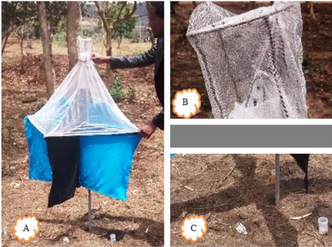
A. Monoconical trap used during study time. B. Flies caught in the cage of trap C. bottles filled with odor attractants (Top: cow's urine, Left: octenol, Right: Ethanol)
