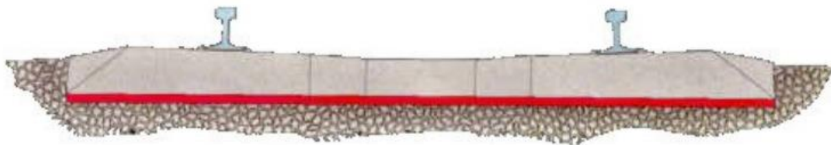
Figure2: Typical construction of a ballasted track [13]
