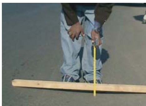
Figure 2.8 Depression from site survey & severity level as per (GTC, 1998)
