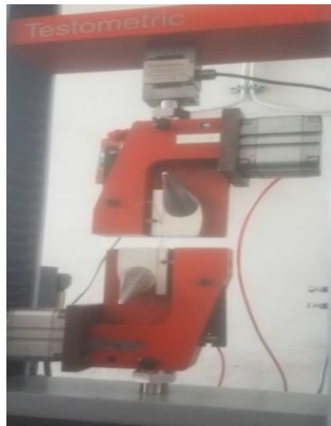
Figure 3.5: Testometric universal testing machine
