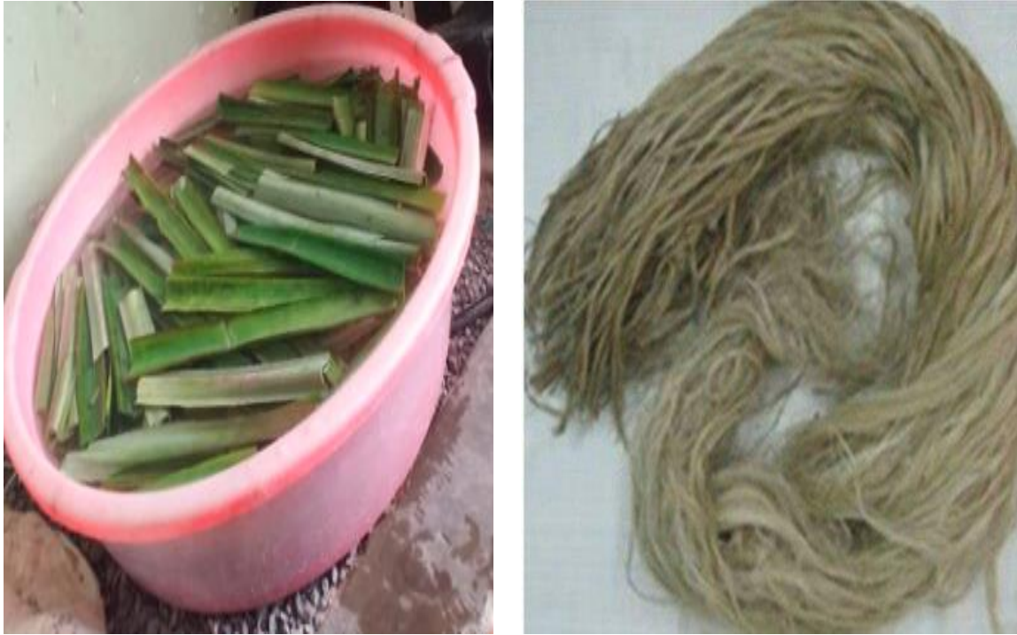
Figure 3.6: Soaking and retting extracting Pineapple leaf fibers
