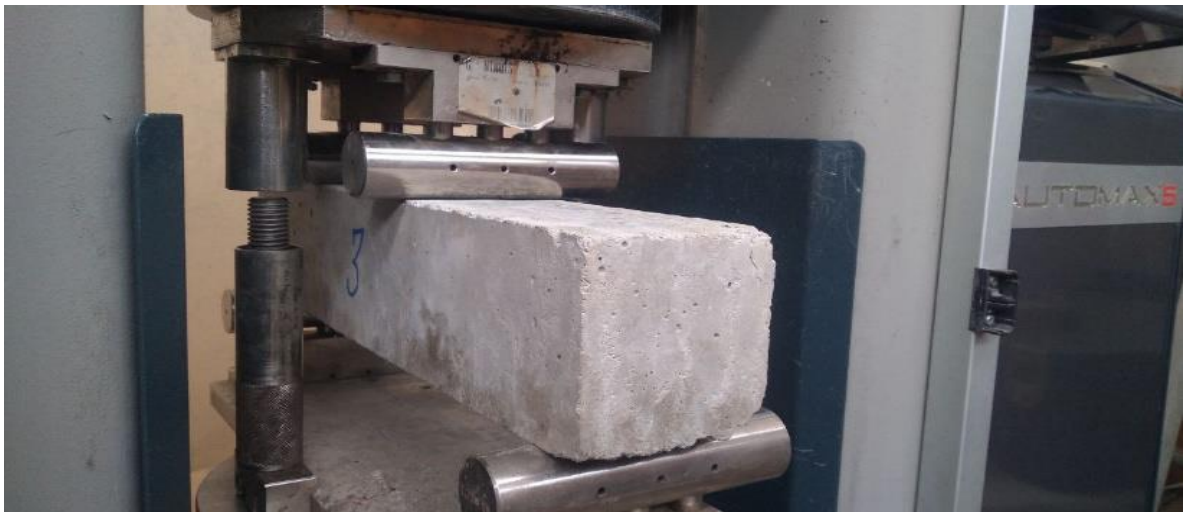
Figure 3.13: Flexural Strength Test Setup
