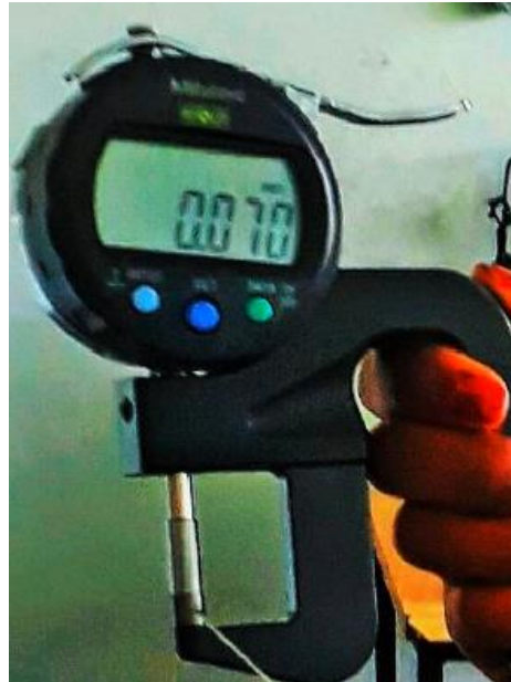
Figure 3.4: Diameter of PALF Using Caliper
