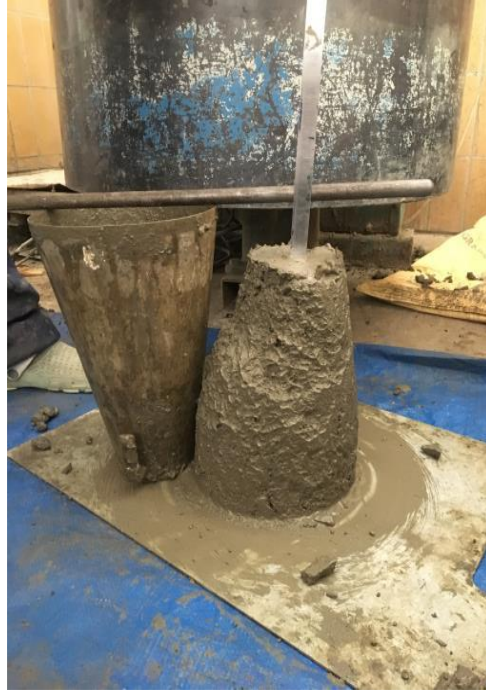
Figure 3.9: measuring slump of fresh concrete mix
