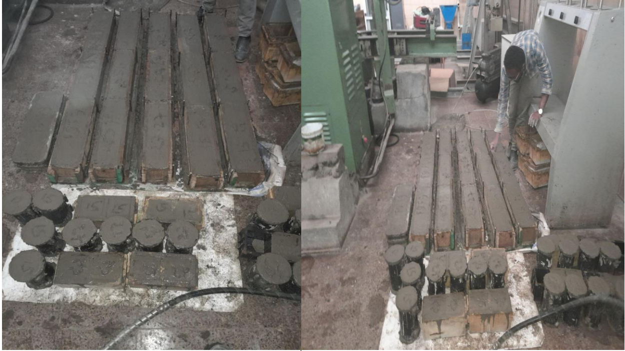
Figure 3.10: Concrete Specimen after cast
