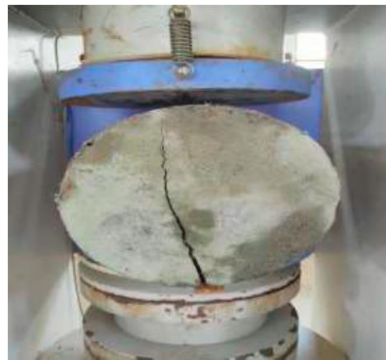
Figure 2.9: Testing of PALF reinforced Cylinder
