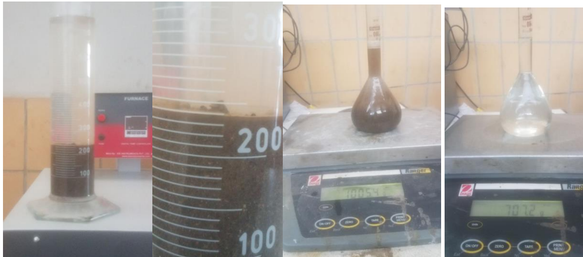
Figure 3.2: Silt content and specific gravity of fine aggregate
