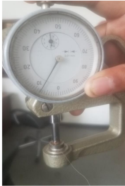
Figure 3.4: Diameter of PALF Using Caliper
