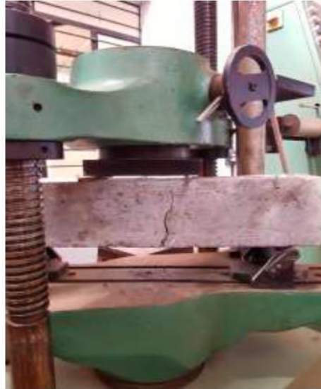
Figure 2.7: Testing of PALF reinforced beam
