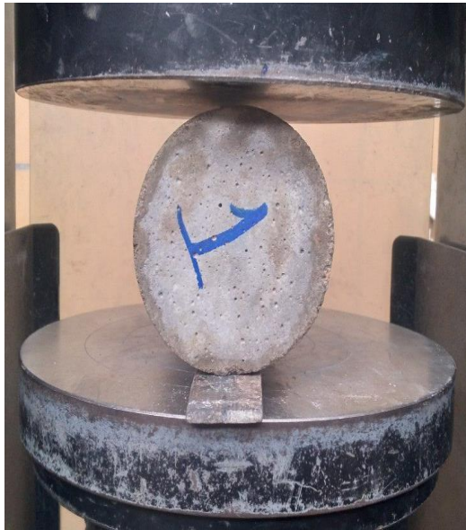
Figure 3.12: Splitting Tensile Strength Test Setup
