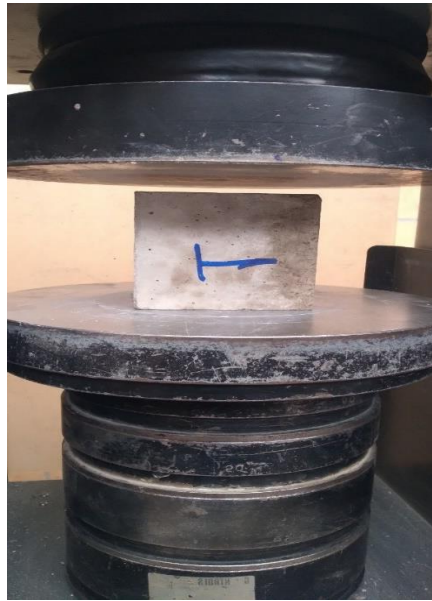
Figure 3.11: Compressive Strength Test Setup
