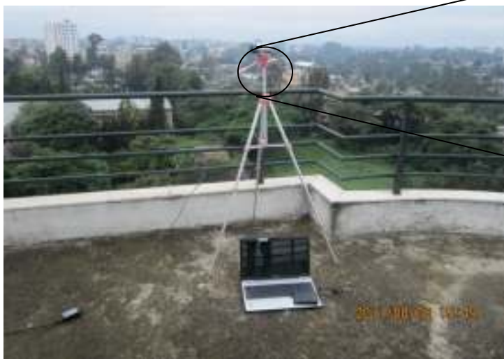
Figure 4: Typical Arrangement of Video camera during recording @ Haile G/Silase building
