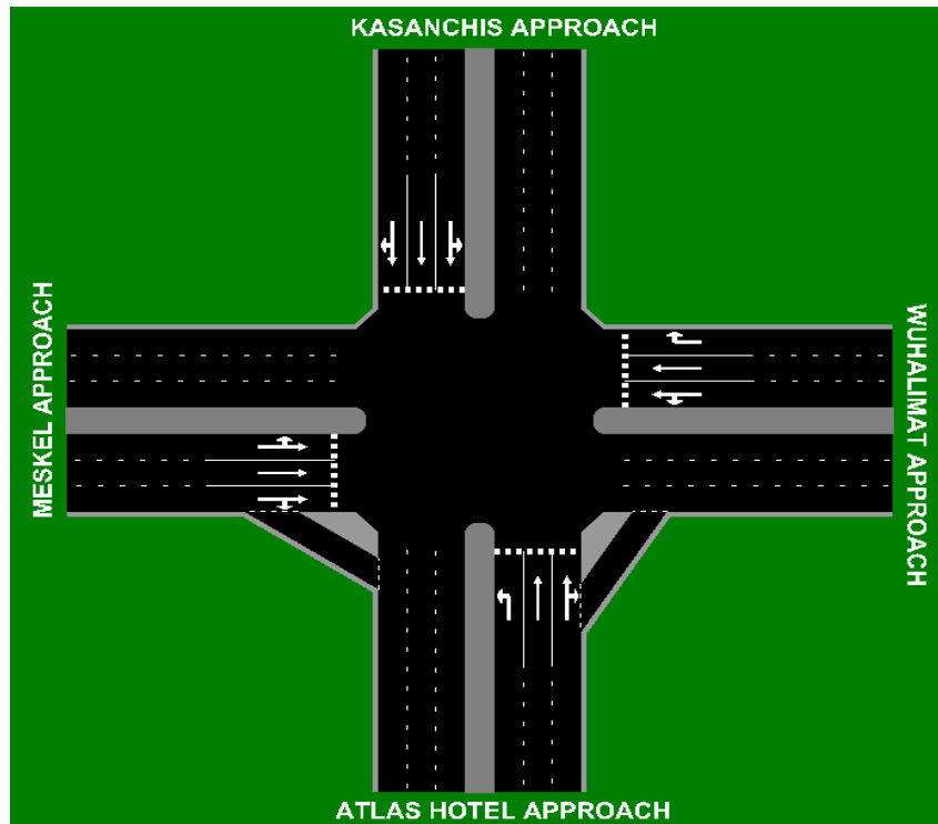
Figure 56: URAEL Intersection Geometry using aaSIDRA
