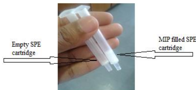
Figure 4.5. 12. Extraction of selected pharmaceuticals using MIP as an adsorbent in SPE cartridge
