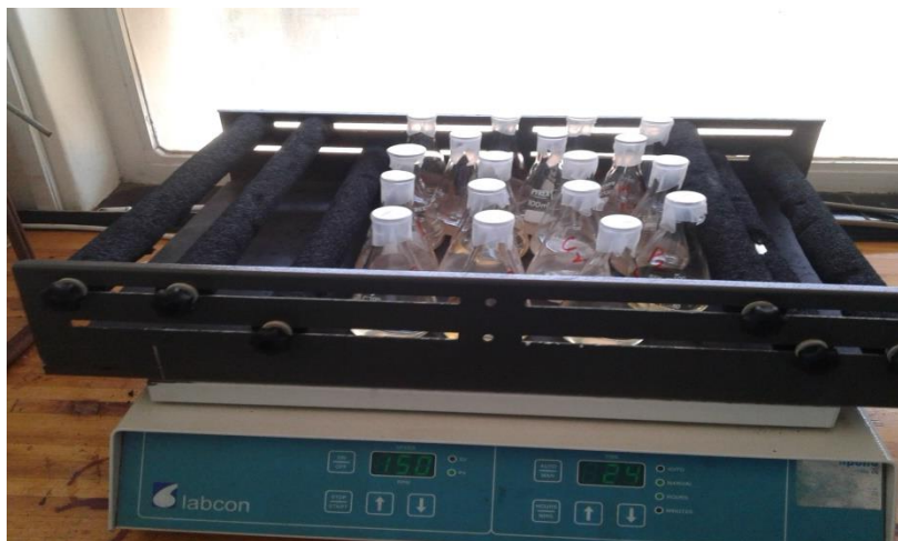
Figure 3.7. 3 Batch adsorption study set up for the removal of pharmaceuticals
