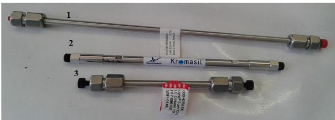
Figure 4.1. 1. Type of chromatographic column used in this study for separation (1- Water Spherisorb phenyl; 2- Kromasil C 18 ; 3- Luna C 18 ).
