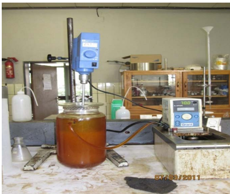
Figure 3.5 Experimental set-up for degumming of crude oil.
