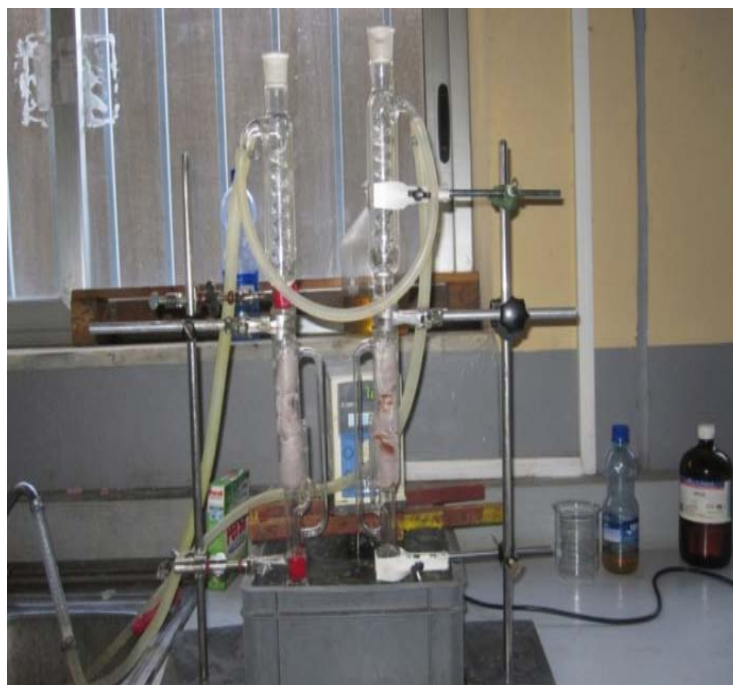
Figure 3.3 Experimental set-up for Soxhlet Extraction
