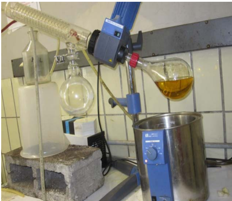
Figure 3.4 Rota vapor used to separate the hexane from the extracted wado seed oil
