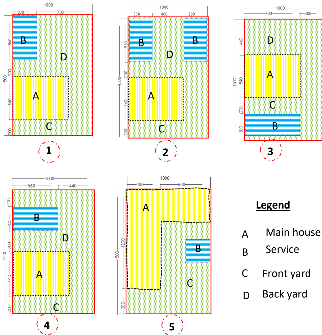
Figure 5.1. Types of Awra Amba compound arrangement.
