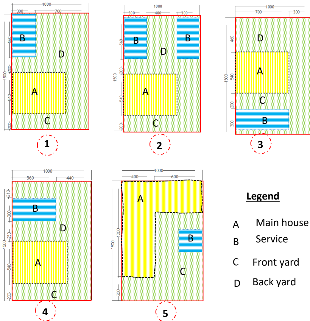
Figure 4.112. Types of Awra Amba compound arrangement.
