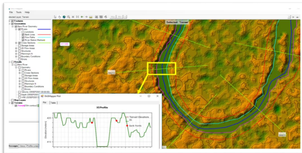
Figure 4-25: Baro River with terrain data and shade of contour interval 20m
