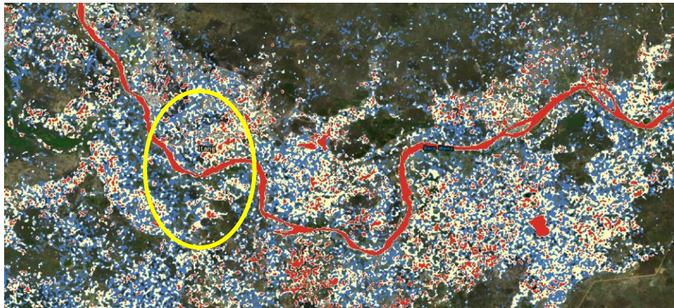
Figure4-42: Flood prone area for the next 20-years (2030-2039)
