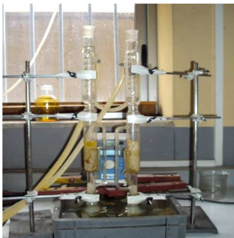
Figure3.1: Laboratory setup of soxhlet extraction unit
