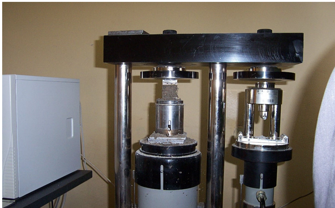
Fig 3.17 Mortar prism tested for compression
