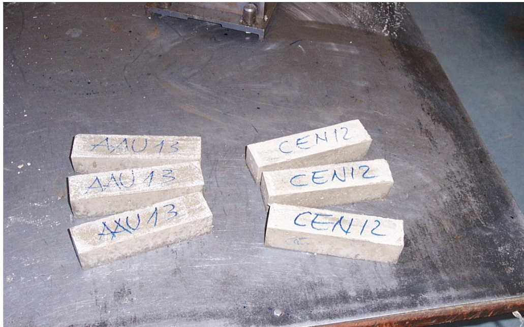
Fig 3.13 Demoulded mortar prisms
