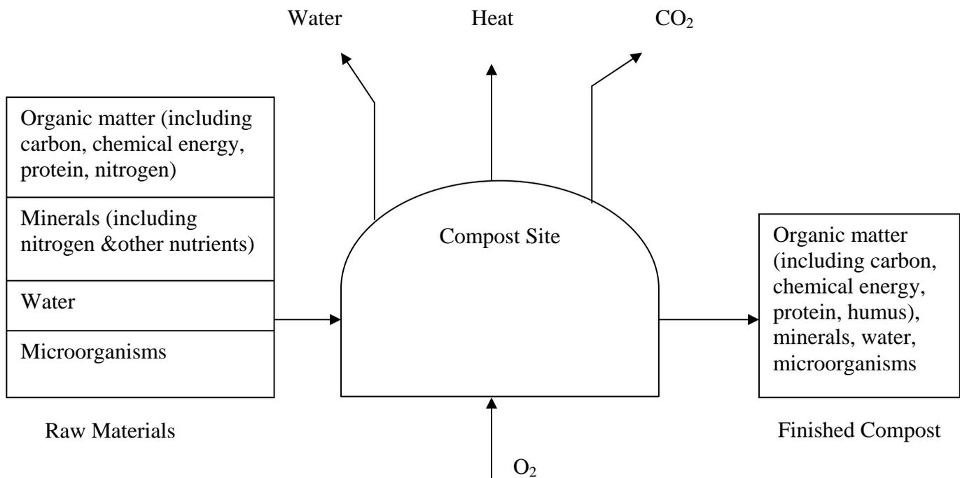
Figure 2.3: Aerobic composting process for organic wastes
