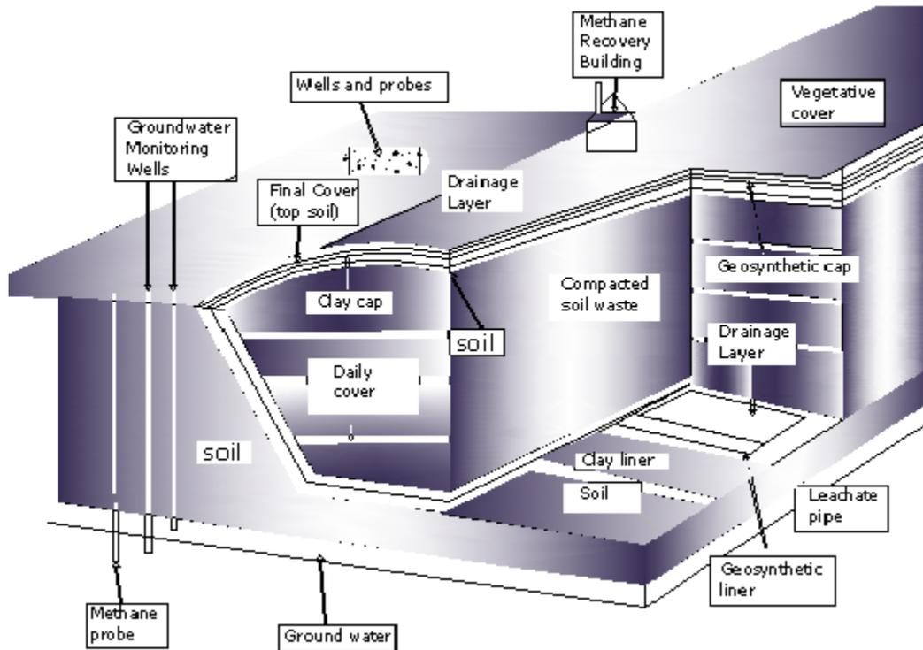
Figure 2.2: Schematic for a typical MSW landfill
