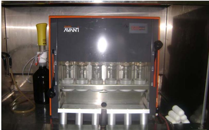
Figure 3.9 Soxtec Soxhlet fat extraction apparatus
