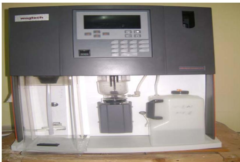
Figure 3.8 kejeltic analyzer unit
