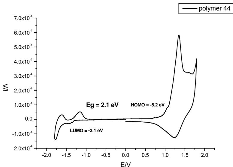
Figure 4: Cyclic voltammogram of polymer **44**.
