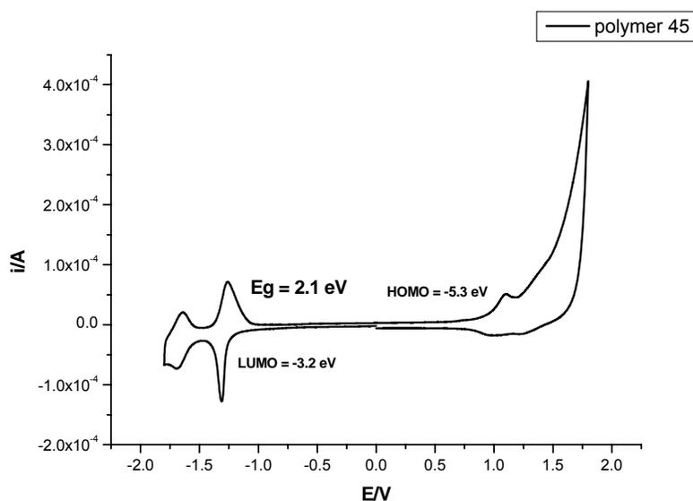
Figure 5: Cyclic voltammogram of polymer **45**.
