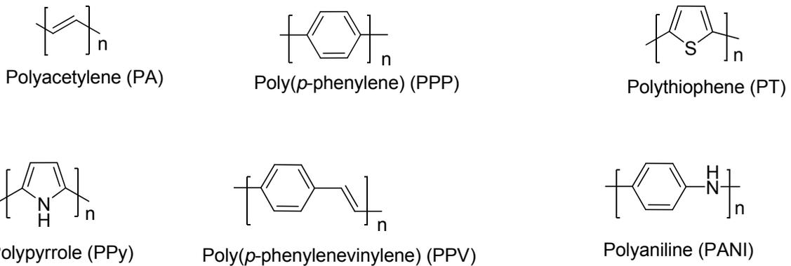
Fig 1: Structures of some conjugated polymers.
