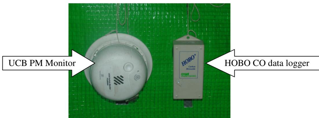
As the manufacturer of the instrument indicated, the CO sensor is temperature compensated over the entire operating range; however, there may be an additional error that increases as the temperature gets farther from 20°C. For temperatures from 0°C to 20°C the readings may be lower by as much as 5% or 5ppm. For temperatures from 20 °C to 40 °C the readings may be higher by as much as 5 % or 5ppm.
