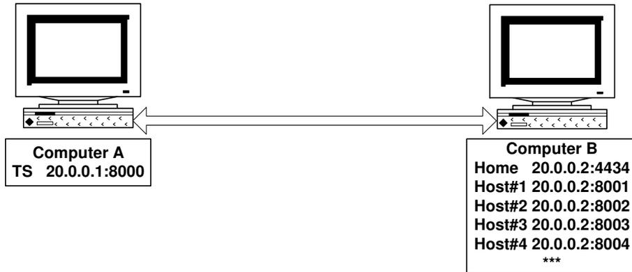
Figure 5.8 Test environment set up
