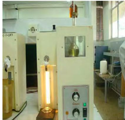
Petroleum products distillation apparatus
