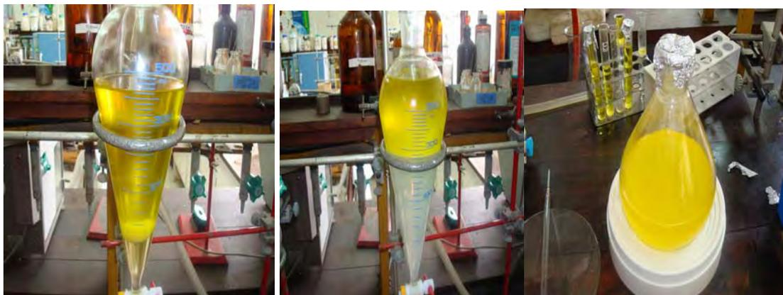
Figure 7. During phase separation      Purification stage      Purified Moringa biodiesel
