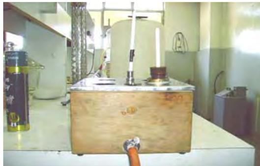
The Peltier device apparatus
