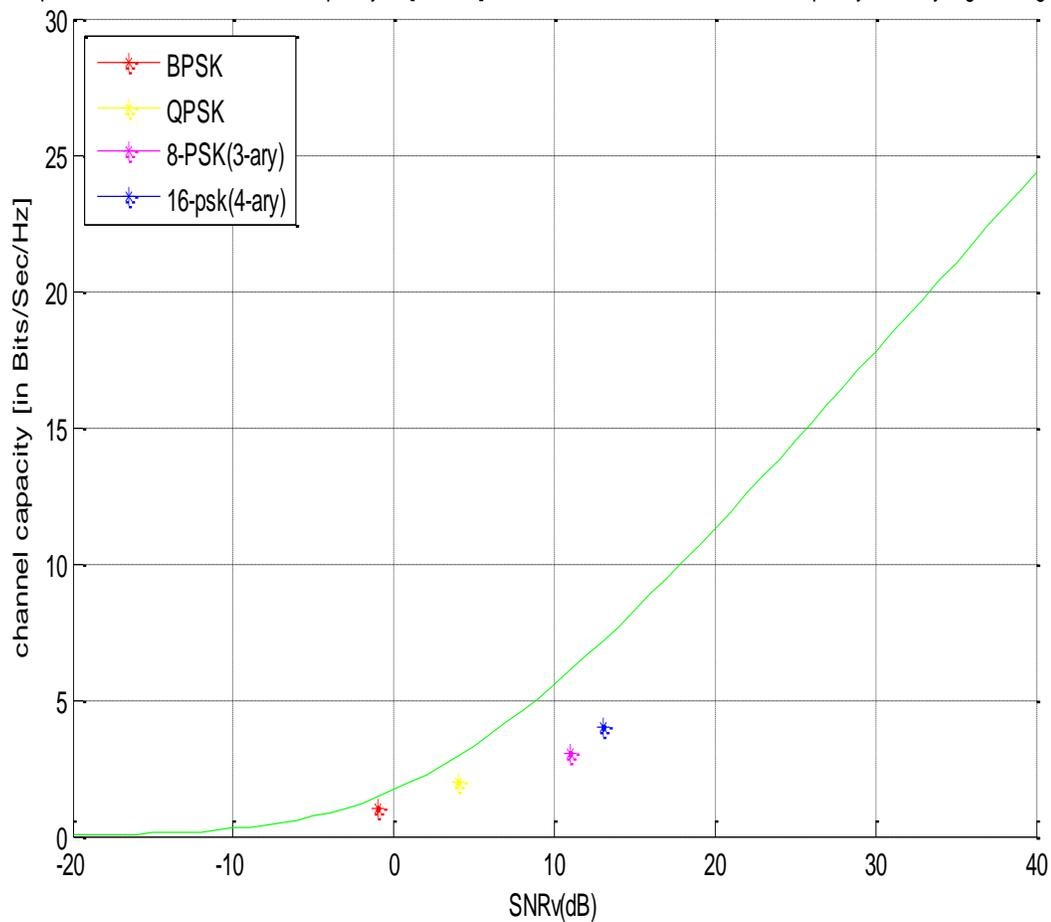
Figure 4-5 A comparison of Gaussian Rayleigh fading channel capacity with Alamouti's channel capacity
