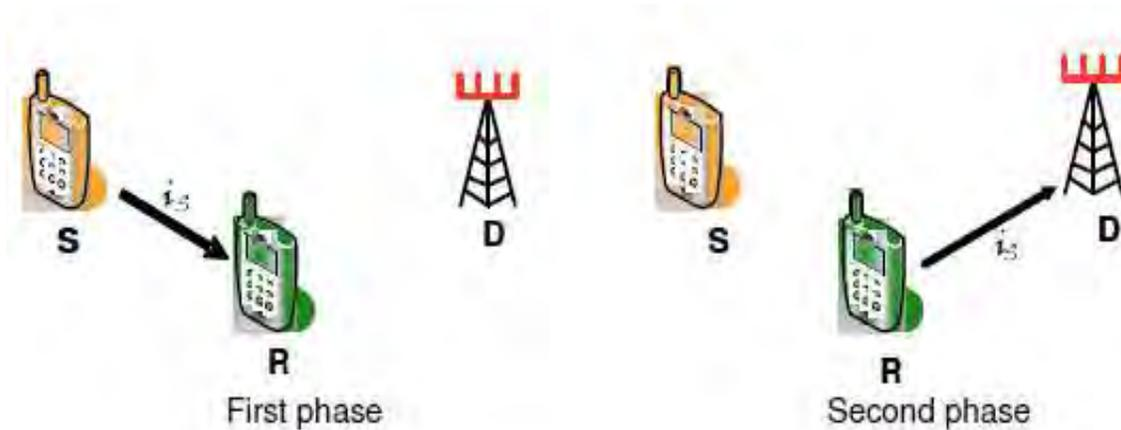
Figure 3-2 Relay-channel system in the uplink of the mobile communication system, where S, R, and D stand for the source, relay, and destination, respectively, and  $i_s$  is the message of the source [11]
