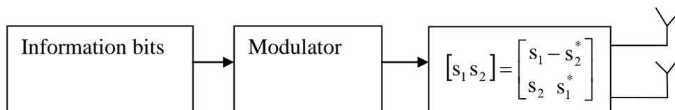
Figure 3-3 A block diagram of Alamouti space time encoder
