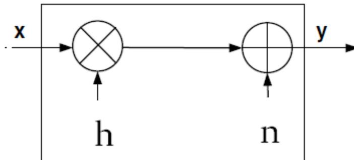
Figure 2-3 Channel model with fading coefficient  $\mathbf{h}$  and noise  $\mathbf{n}$ .
