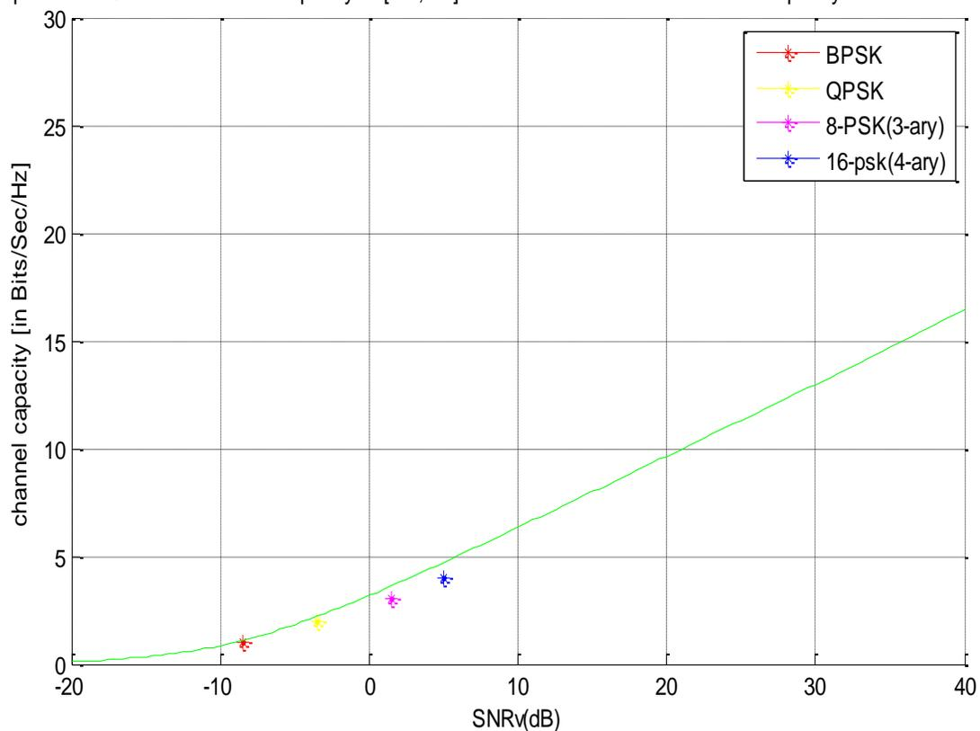
Figure 4-6 A comparison of Gaussian Rician fading channel capacity with Alamouti's channel capacity
