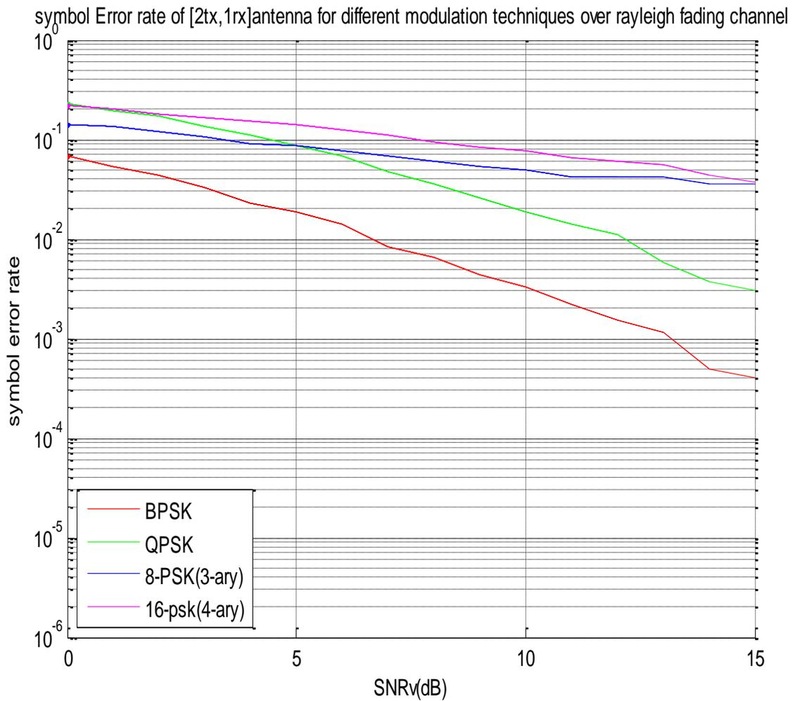
Figure 4-4 The SER performance comparison among BPSK, QPSK, 3-PSK and 4-PSK
