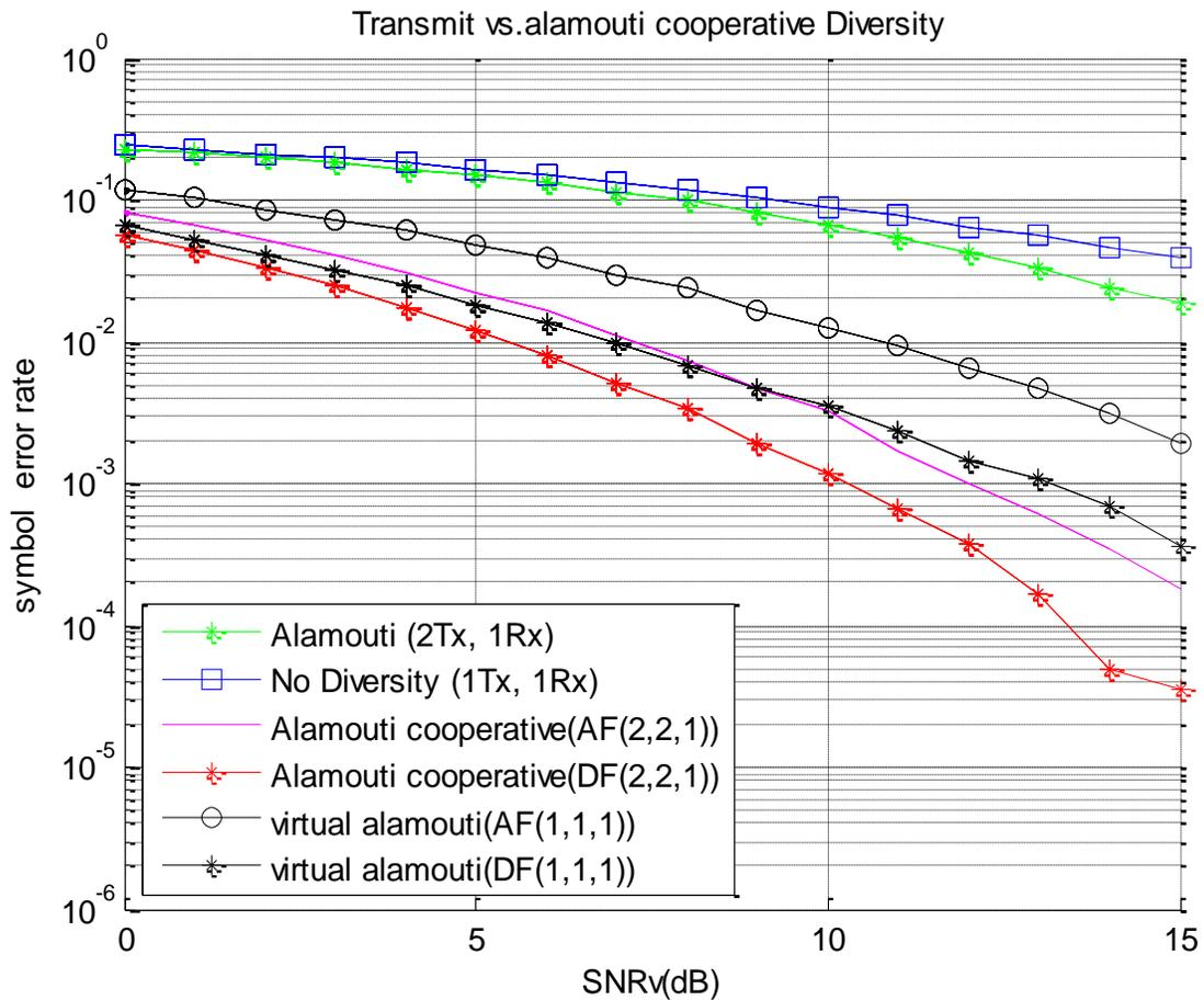
Figure 4-3 SER performance comparison of different systems when the direct down link channel is -10dB
