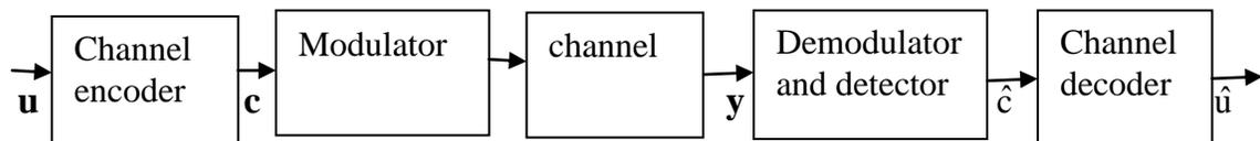
Figure 2-4 System model of point-to-point transmission
