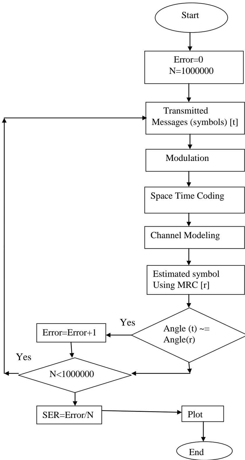
Figure 4-1 Flow chart for the simulation
