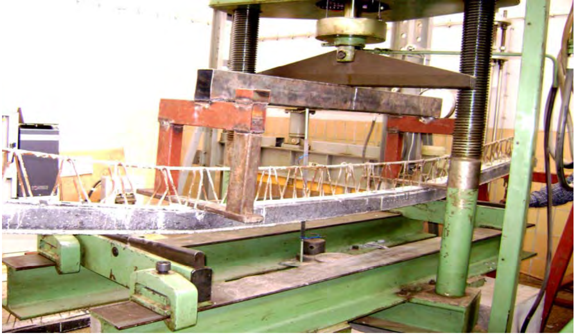
Fig.2.1 Bending Test Setup
