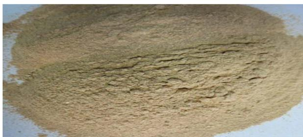
**Figure 2:** Powdered orange peel sample used for dye adsorption
